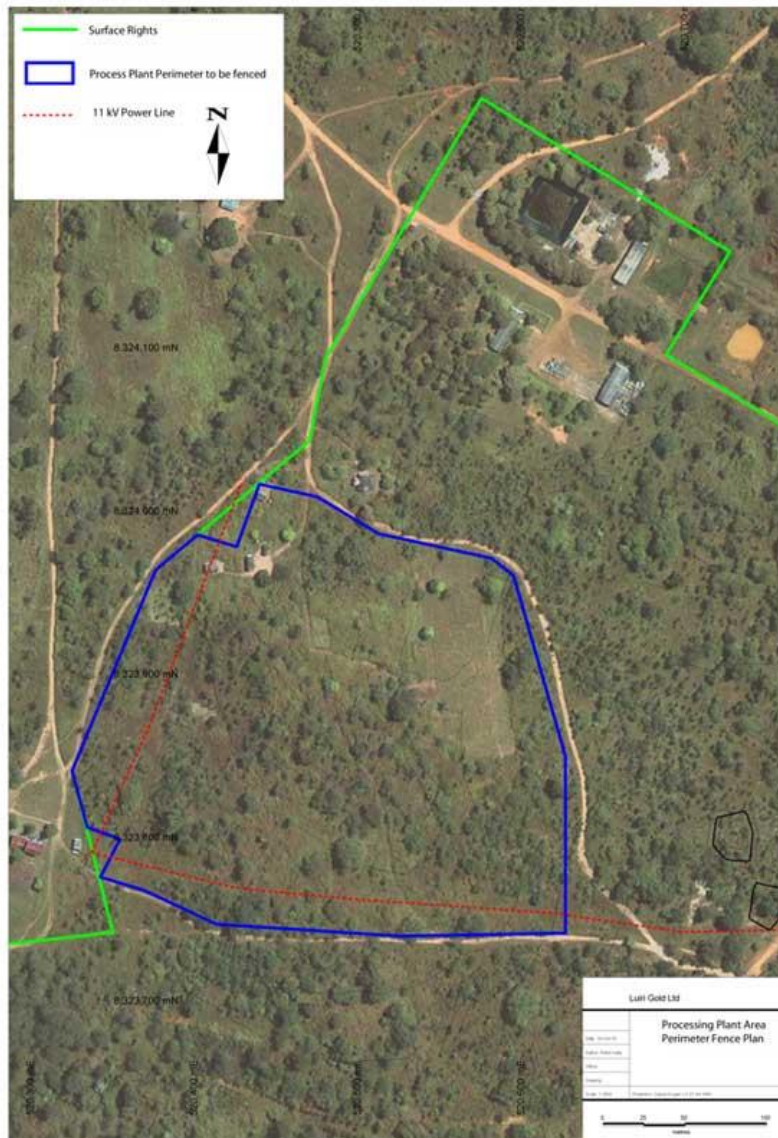
Figure 5 - Zambian Process Plant Ground Clearance and Fencing
